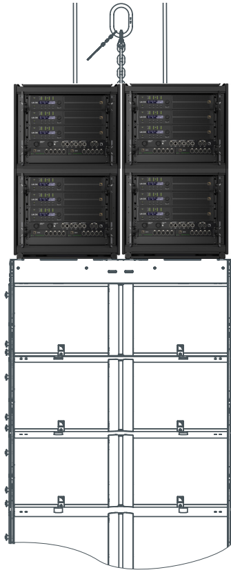
Stacking onto K1-BUMP (max. 4 LA-RAK II + 24 K1)
